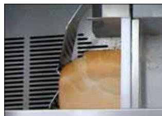
Through the slotted openings the crumbs fall directly into the easily removable tray.
