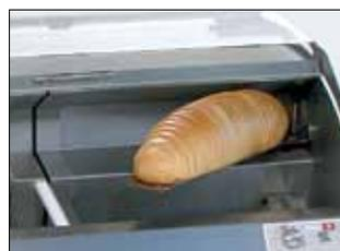
The bagging scoop can also be fixed above the infeed chute if required.
